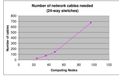
•Flat networks with small switches don't scale well to large
